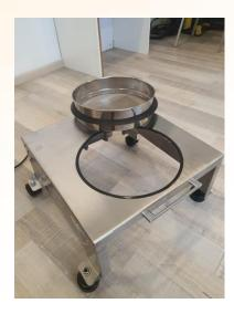
The Vibro Sieve offers a quick solution to mechanically separate out larger particles or impurities from the paste or liquid foods that you may be processing. Ideal for all types of cocoa, oils, butters, nut butters, batter etc..
